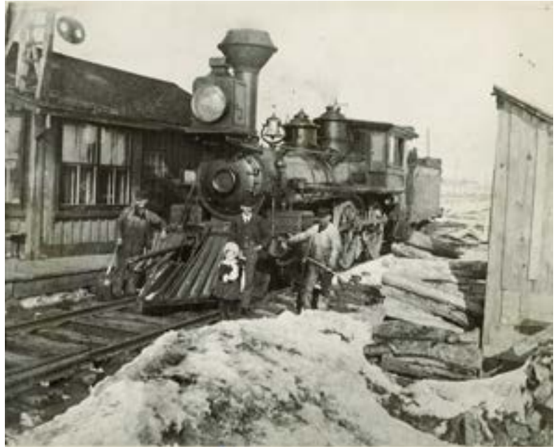
This engine was often at Orangeville and would help other trains up inclines, such as Caledon Mountain. There is also cordwood on the right used for fuel. Photograph was taken at Melville Cross station, ca. 1900. MoD Collection, P-2577.
