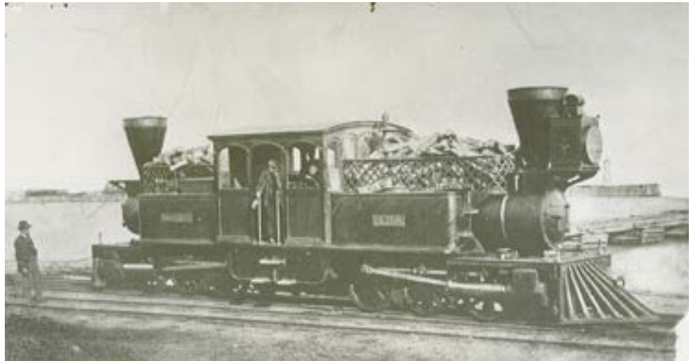
Steam engine, the 'Caledon' at Orangeville in 1872. It was a double-header engine used by the TGBR but was scrapped after the gauge size was changed. It was not able to do the work it was built for, such as take heavy cargo up Caledon Mountain. MoD Collection, P-2574.
